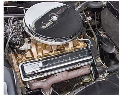
NASCAR racer and engine builder Smokey Yunick may have had a hand in preparing engines, including the V-8 now in the restored car—a 307-cid version of the original 265. It is a true 1955 engine, as it's fitted with early exhaust manifolds and does not have an oil filter.
