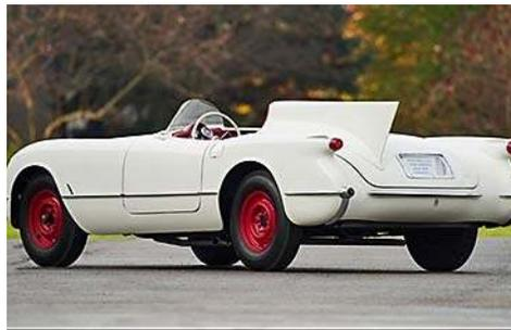
While in initial testing, the car's appearance remained showroom stock. But after being assigned to Duntov it was fitted with a minuscule windshield, a cockpit tonneau cover over the passenger's seat and a tall fin meant to improve stability. A build order of Nov. 7, 1955 was signed by Duntov requests reworking of the body, engine, transmission and rear
