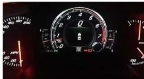
and 4,500 rpm. During the engine break-in period, please try to shift gears between those guides and ignore the 6.2-liter LT1 V8 engine's 6,500 rpm redline if you want a trouble-free Corvette with a manual.
