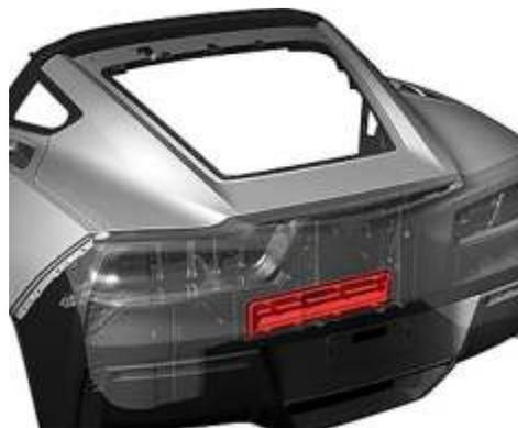
below the hatch door. When you open the hatch, current is sent to a nickel-titanium alloy wire that causes the cabin pressure relief valve to contract and open its vents. When you close the Chevrolet Corvette's hatch door, the current is removed, and Venetian blind-like louvers close more silently than a puny electric motor doing the same thing. It's intelligent engineering that's hideously underrated.
