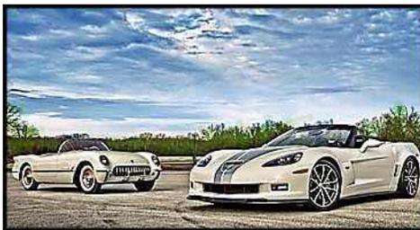
SMC made the bodywork panels smoother and, as a result, the paint finish was improved. All Corvettes constructed since have an SMC body, though once again technology made it possible to alter its composition and make the panels stronger and, at the same time, thinner.
