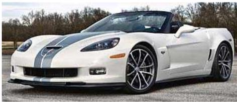
As the name implies, the 427 edition has a 427-cubic-inch LS7 engine borrowed from the Z06, and it's rated at 505 hp and 470 lb-ft of torque. Chevy says this is the most powerful production convertible in Corvette's history. This model will be offered only with a six-speed manual. Carbon fiber is used for the raised hood, the Z06-style fenders and floor panels and as an option for the front splitter and rocker panels.
