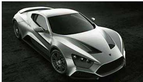
The massive 7.0-liter is being supercharged and turbocharged (hence the initials ST) and tweaked to deliver 1,104 horsepower and 1055 pound-feet of torque roughly twice the output and torque of the stock LS7 powerplant. Fed through a six-speed manual gearbox and a hydraulic limited-slip diff, the bi-fuel engine is electronically governed to hold top speed to 233 mph, with 0 to 60 mph accomplished in a whisker under 3.0 seconds.
