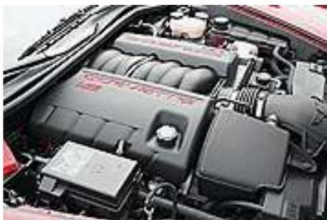
In the engine bay of the C6 Corvette, the new 6.2L LS3 V-8 now cranks out 430 HP @ 5,900 rpm and 424 lb-ft of twisting force @ 4,600 rpm. That's 25 hp more than the pricey and complex Lotus-designed LT5 in the old ZR-1, and the base price of this car starts at about \$45K. At its 2008 model intro, GM offered up a base 'Vette with the six-speed manual gearbox to toss around.
